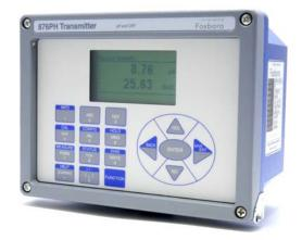
The Foxboro<sup>®</sup> brand Model 876PH is a 2-wire loop powered intelligent transmitter that, when used with appropriate electrochemical sensors, provides measurement, local display, and transmission of pH, ORP (Oxidation-Reduction Potential), or ISE (Ion Selective Electrode) concentration. The transmitter outputs a HART digital signal and a 4 to 20 mA analog output. Versions are available for use with both analog and Smart (digital) sensors.
